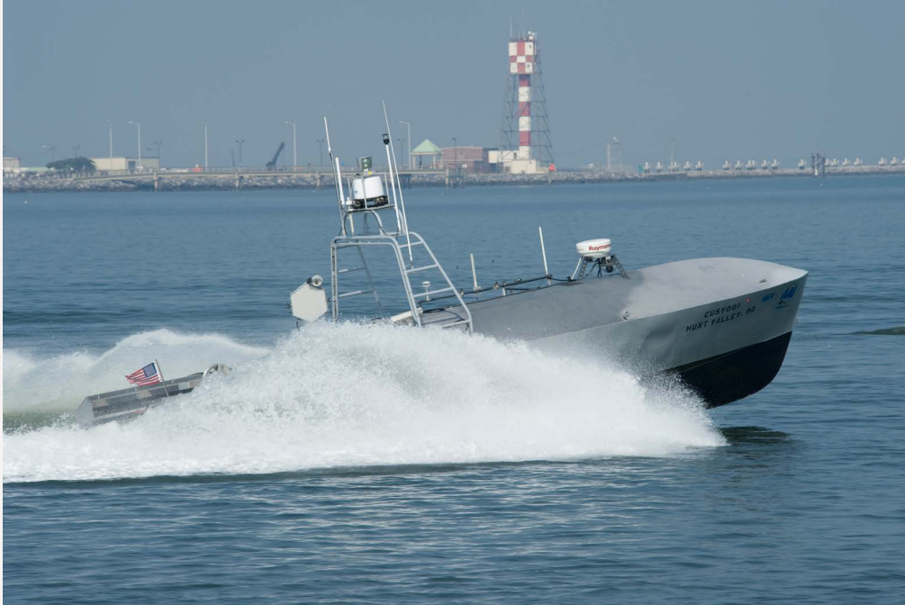
A common unmanned surface vehicle. Photo courtesy US Navy .
